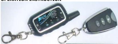
(the left remote is two-way, there're 3 LEDs on the screen: RED, BLUE and YELLOW; the right remote is one-way. )
