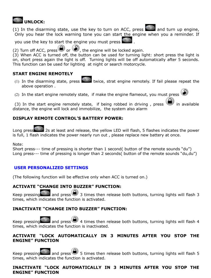
Keep pressing and press 6 times then release both buttons, turning lights will flash 6 times, which indicates the function is inactivated.
